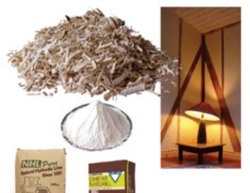
Hemp wood chips or hurds are mixed with lime based binders to create a breathable masonry material called hempcrete, This is used to build monolithic walls and floors and to fill roof cavities.
